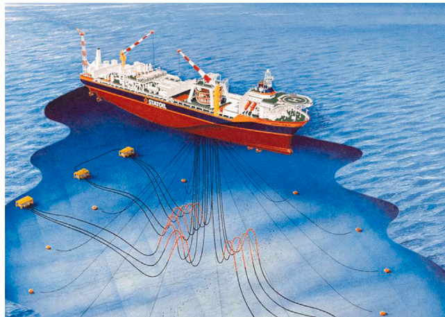
Fig. 3. Illustration of the Norne 6608/10 FPSO. Source: Courtesy: Equinor.
